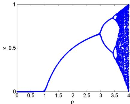
Figure 5: Bifurcation diagram of the dynamical systems (2.1) with  $r = 1$  and (2.3) where  $N = T = 70$ .
