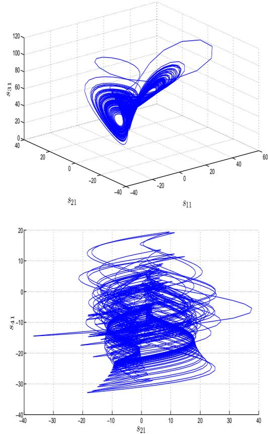
**Figure 2.** Hyperchaotic attractor of Gao system in three dimensional space and in  $s_{11} - s_{41}$  space
