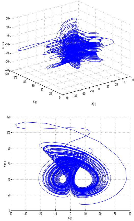
**Figure 3.** Hyperchaotic attractor of Gao system in three dimensional space and in  $s_{21} - s_{31}$  space
