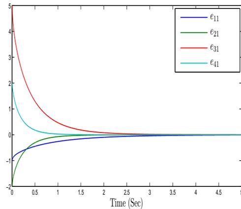
**Figure 7.** Convergence of anti-synchronization errors to zero for integer order Cai system and fractional order Gao system
