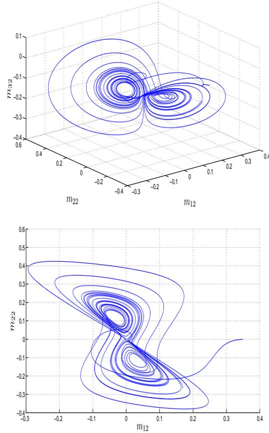
**Figure 4.** Chaotic attractor of fractional order Newton Leipnik system in three dimensional space and in  $m_{12} - m_{32}$  space
